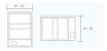
The window installation kit allows you to install the air conditioner in most vertical-sliding windows 18" to 50" wide, or horizontal-sliding windows from 18" to 50" high.
