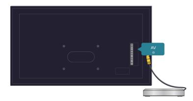
Make sure that the audio cable is connected to the correct audio output connector on the external device.
