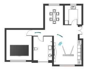
Position your wireless router, modem router, or access point in a central location. Avoid putting it in a corner.
