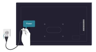
If the signal is intermittent, unplug the TV power cord from AC outlet and re-plug after 60 seconds.
