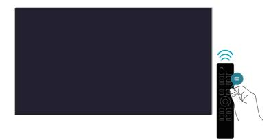
If the TV does not respond with the Bluetooth remote control, try pairing the remote control to the TV by pressing and holding the 🕞 and 🎧 button at the same time.
