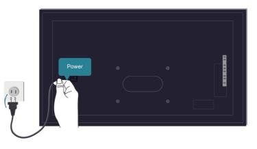
Unplug the TV power cord from AC outlet and re-plug after 60 seconds.
