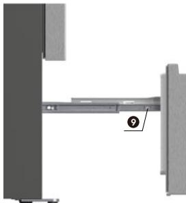
5. Pull out the freezer door and lift it up in the direction of the arrow.
