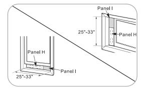
For window openings from 25" to 33", use the window vent panel(Panel H) and a extension panel (Panel I).
