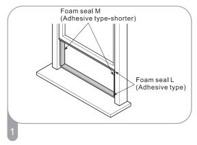
Cut the foam seal L(adhesive type) & M (adhesive type-shorter) to the proper length, and attcah it to the window sash and frame.
