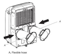
5. Confirm the hose is locked in place before operating.
