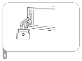
Insert the diffuser into the opening in the vent panel and slide it to lock it into place.
