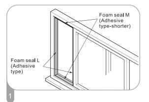
Cut the foam seal L(adhesive type) & M (adhesive type-shorter)to the proper length, and attach it to the window sash and frame.
