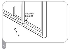
Install the Window-lock bracket with a type F screw as shown if you need.
