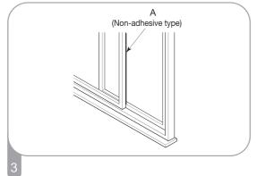
Cut the foam seal A(Non-adhesive type) to the window width. Stuff the foam seal A between the glass and the window to prevent air and foreign objects from getting into the room.
