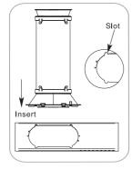
Align the tabs on the diffuser with the slots in the vent panel. Insert the diffuser into the opening in the vent panel.
