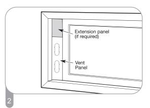
Insert the vent panel assembly, including extension panels, if needed, into the window opening. Extend the extension panels, if used.
