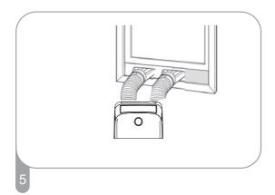
Insert the diffuser into the opening in the vent panel and slide it to lock it into place.
