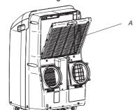
A.Evaporator air intake fliter panel door
