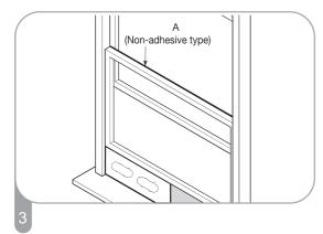
Cut the foam seal A(Non-adhesive type) to the window width. Stuff the foam seal A between the glass and the window to prevent air and foreign objects from getting into the room.
