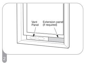
Insert the vent panel assembly, including extension panels, if needed, into the window opening. Extend the extension panels, if used.
