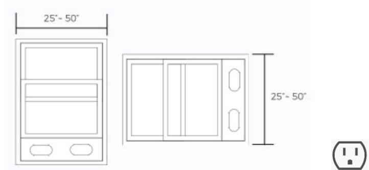
The window installation kit allows you to install the air conditioner in most vertical sliding windows 25" to 50" wide, or horizontal-sliding windows from 18" to 50" high.
