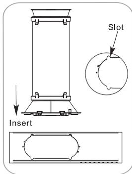
Align the tabs on the diffuser with the slots in the vent panel. Insert the diffuser into the opening in the vent panel.
