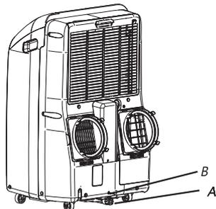
A.Primary drain cover B.Primary drain plug
