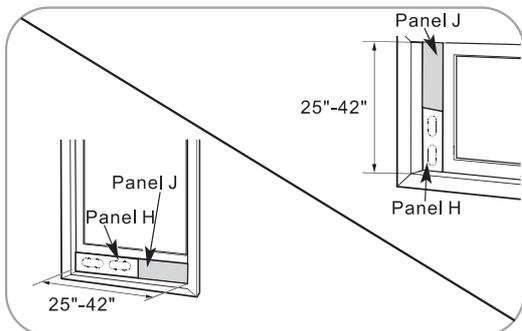
For window openings from 25" to 42", use the window vent panel (Panel H) and a extension panel (Panel J).
