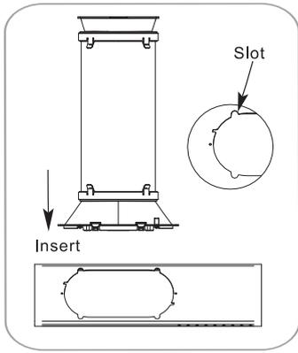
Align the tabs on the diffuser with the slots in the vent panel. Insert the diffuser into the opening in the vent panel.
