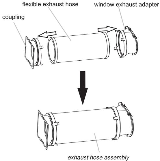
3. Insert the coupling into the slot on the back of the air conditioner.
