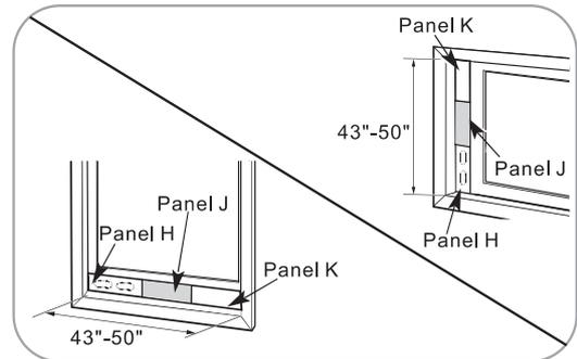
For window openings from 43" to 50", use the window vent panel and two extension panels (Panel K and Panel J).
