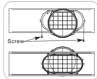
Insert the screw in the hole in the diffuser to prevent the diffuser from sliding out of the vent opening.
