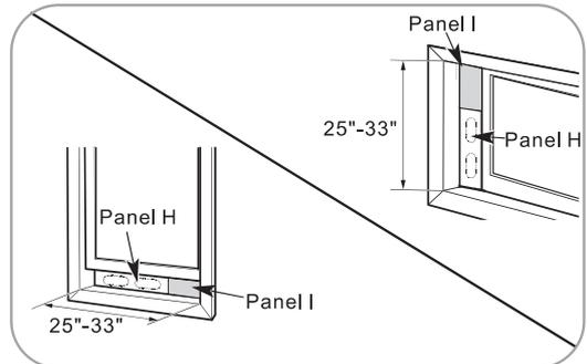
For window openings from 25" to 33", use the window vent panel (Panel H) and a extension panel (Panel I).
