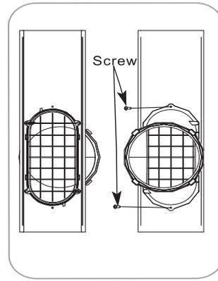
Insert the screw in the hole in the diffuser to prevent the diffuser from sliding out of the vent opening.
