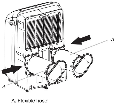
5. Confirm the hose is locked in place before operating.
